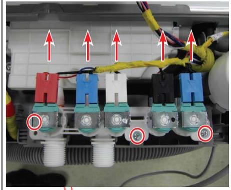
1. Check the resistance for the water supply valve.
