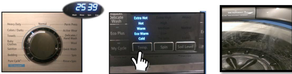
**Step4.** Press the **Temp Key** to turn on the water valves. After turning the water valves on the displayed number should drop. With no water the number will be between 2550 – 2600. If you leave the valves running the number will stop around 2400. After the water is shut off (including any dripping), the number should eventually stop moving..
