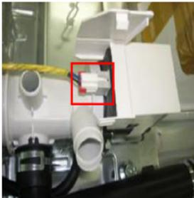
Resistance : Approximately 174Ω between the terminals for the Water Supply Valve.
