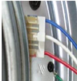
Plug out the connector and read resistances at any two of the three terminals on Motor
