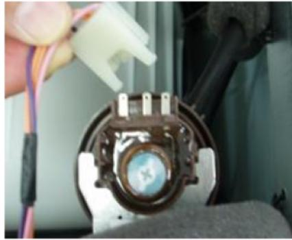
1. Check the water level sensor frequency.
