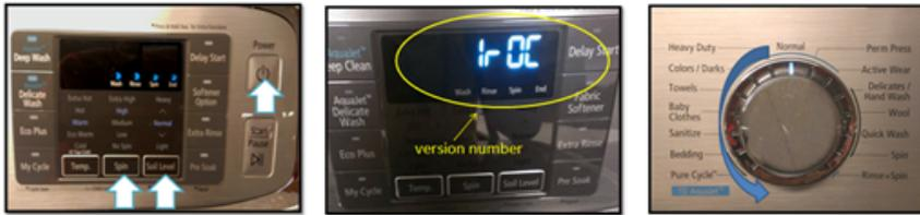
**Step3.** Put the setting into Colors / Dark, a 4 digit number will be displayed as shown in the image below.
