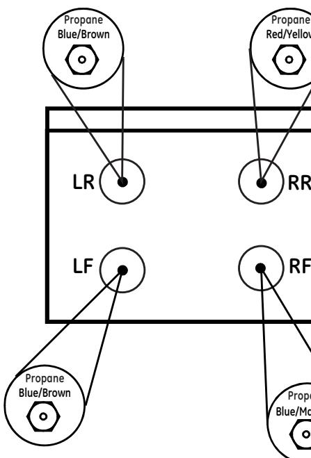
To prevent leakage, make sure the orifices are securely screwed into the gas supply tubes.
