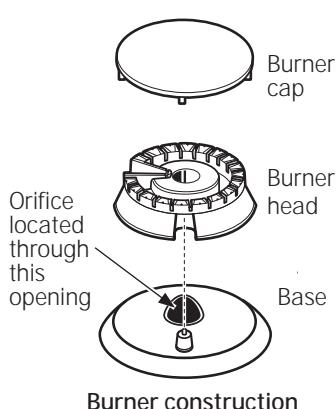
5. Using a 7 mm or 9/32" nut driver, remove the top burner orifices. These may be accessed through the burner opening in the base.
